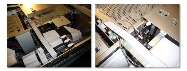
Put the CRT shield and flat cables back in place. To try the mod, depress the ENHANCED ACCURACY or HARDCOPY button before power on and release it about two seconds after.
