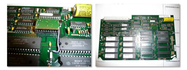
Prepare a 66cm long (from memory, I may be wrong) twin wire with a 2-pin 100mil-pich connector end. Prepare the other end with 2-mm long tinned tips. Unscrew the A11 front panel board and solder the two wires to the pictured solder pads of the flat wire connector. Put the panel back and route the wires as displayed. Attach the connector to the module and sit the A18 board back in place.
