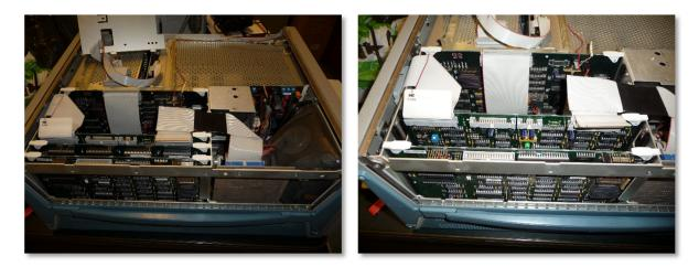
Remove U440 from its socket. Check its orientation is correct like in the picture here.
