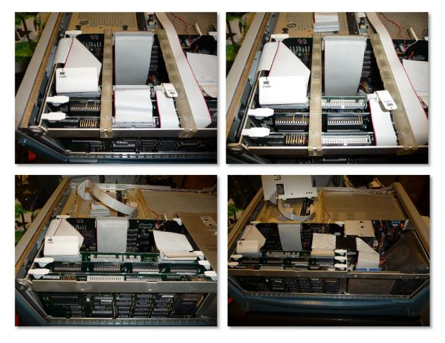
Remove the CRT cover (2 small Torx screws on the mainframe side and one larger Torx screw near the top center of the cover). A18 may then be removed for FW and mod installation.
